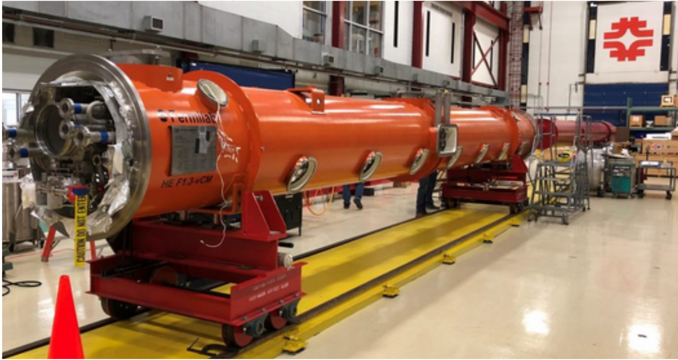
cryomodule at FNAL, destined for LCLS-II @ SLAC
